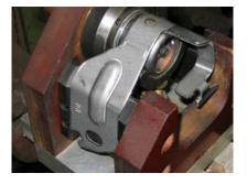
Figure 3 Hydraulic Motor Face Plate
