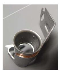
Figure 5 Airbag Component: Photograph Brazed Airbag Detail
