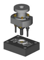
Illustration: Press Assembly Tool to Facilitate a "Press-Fit"
