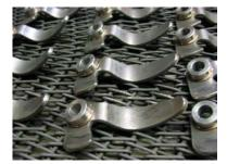
Lever Photograph of Copper Braze Rind pre-placed in Position for Furnace Brazing
