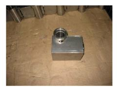
Hydraulic Valve Body Photograph of GTAW [Tig Weld] Required to Hold Parts In Position for Furnace Brazing
